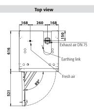
Diagram shows left-hinged door. Dimensions are identical for a right-hinged fitting.
