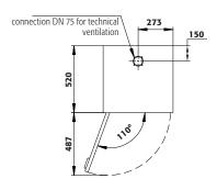
Diagram shows left-hinged door. Dimensions are identical for a right-hinged fitting.
