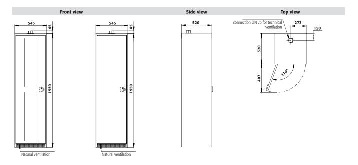
Diagram shows left-hinged door. Dimensions are identical for a right-hinged fitting.
